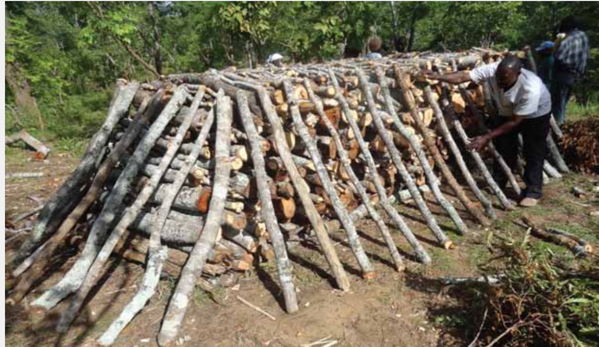
Preparing an improved basic earth kiln (IBEK) in Kilosa. IBEKs increase the efficiency with which wood is transformed into charcoal.
